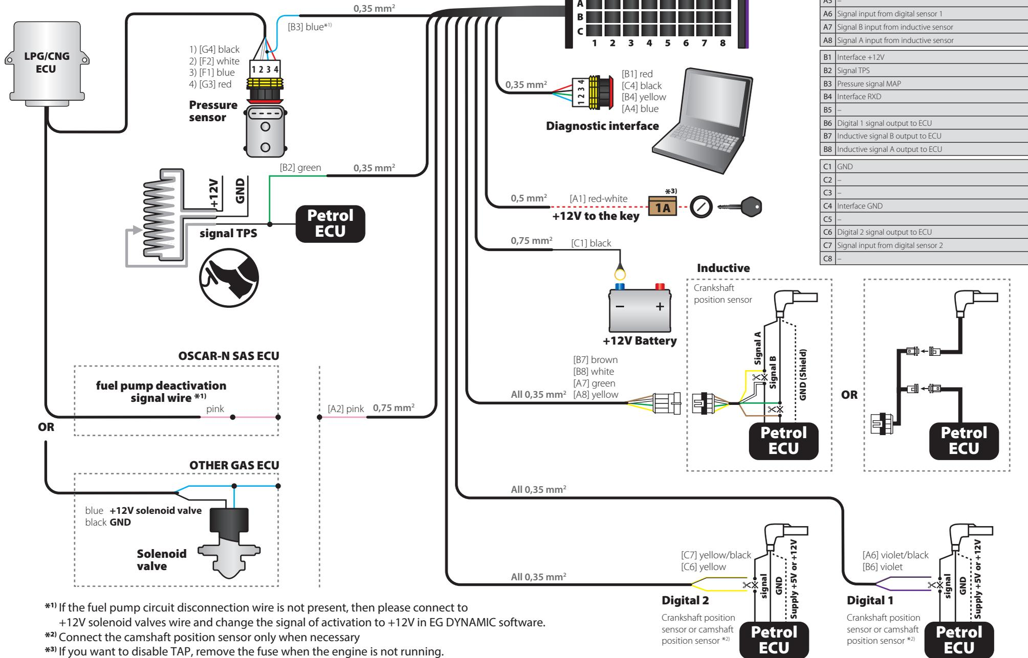
\*<sup>1)</sup> If the fuel pump circuit disconnection wire is not present, then please connect to +12V solenoid valves wire and change the signal of activation to +12V in EG DYNAMIC software.
